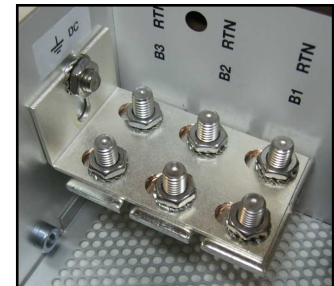
Fig. 9b – Grounded Common Return (zone B)
