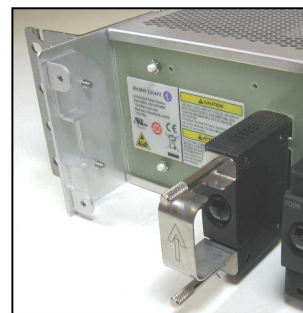
Fig. 13a – Removal tool applied to breaker
